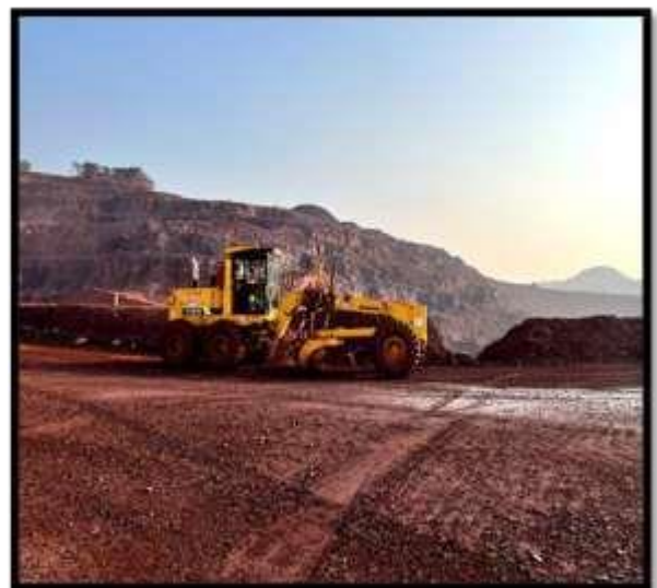
DOZER AND GRADER AT WORK MAINTAINING HAUL ROAD CONDITION
